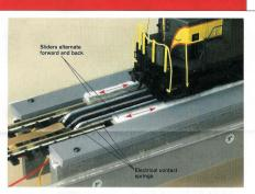
be used with traction tires.) A Faulhaber motor drives the cleaning sliders through a pair of cams.
